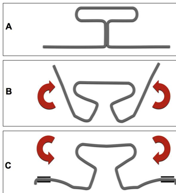
**Fig 2.** A, TLS in passive form; B, TLS preactivated by concentrated bends; C, TLS engaged in brackets (loaded in the opposite direction to preactivation).
